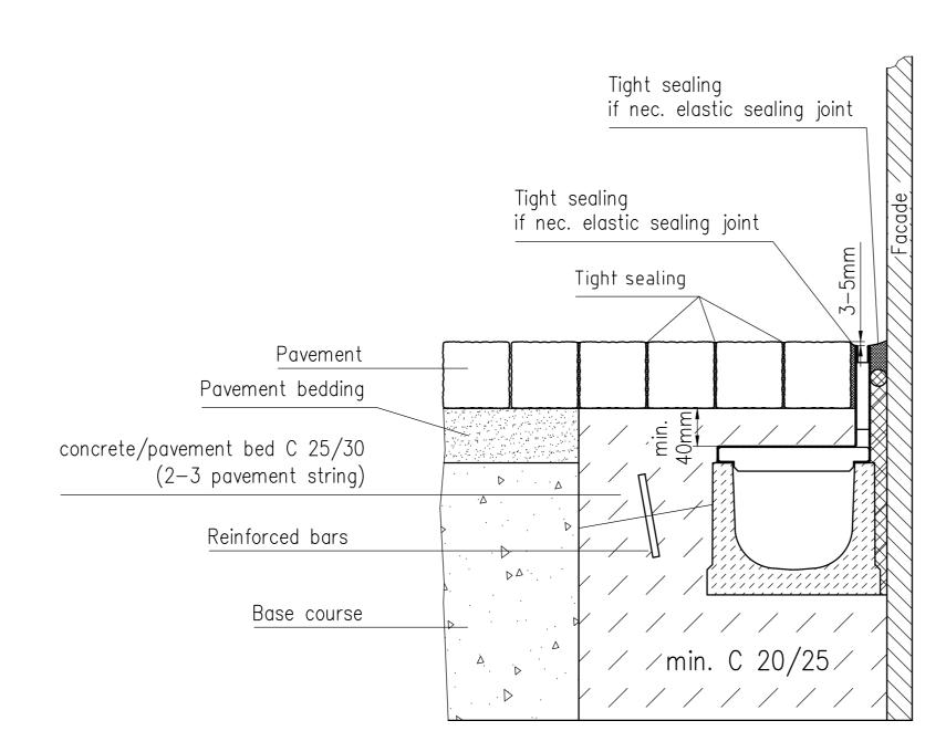
Constructed in accordance with local specifications using non-settling frost-free sub-bases (E.g. RSTO)
