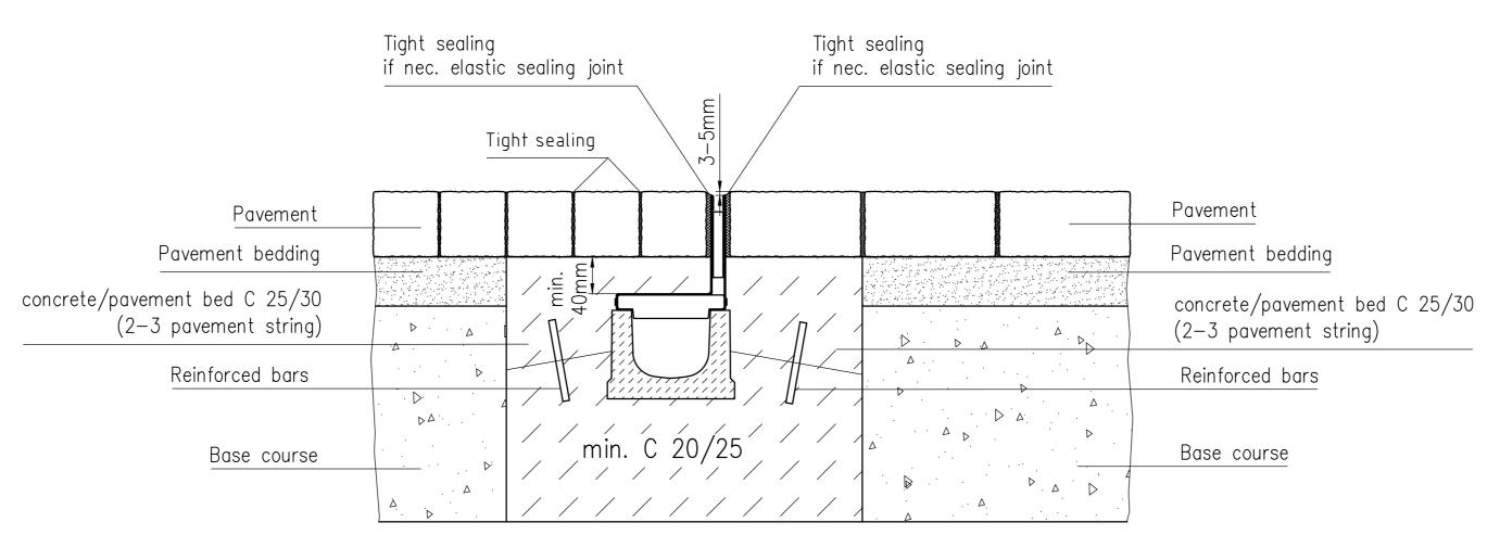
Constructed in accordance with local specifications using non-settling frost-free sub-bases (E.g. RSTO)
