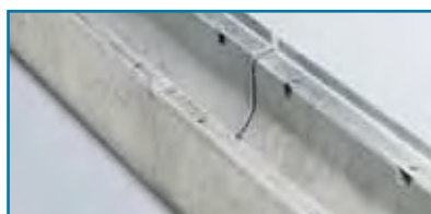
1. Channels groove at the tongue – prior to jointing
